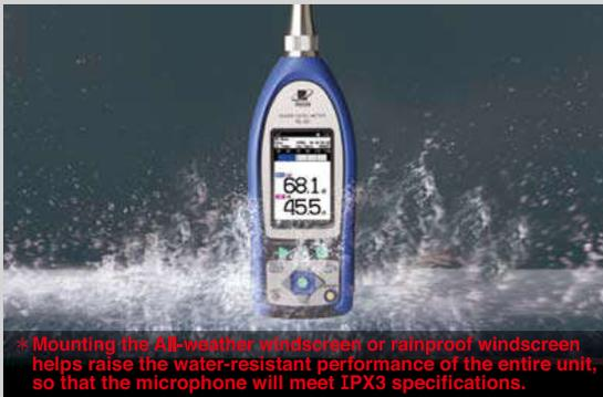
\* Mounting the All-weather windscreen or rainproof windscreen helps raise the water-resistant performance of the entire unit, so that the microphone will meet IPX3 specifications.
